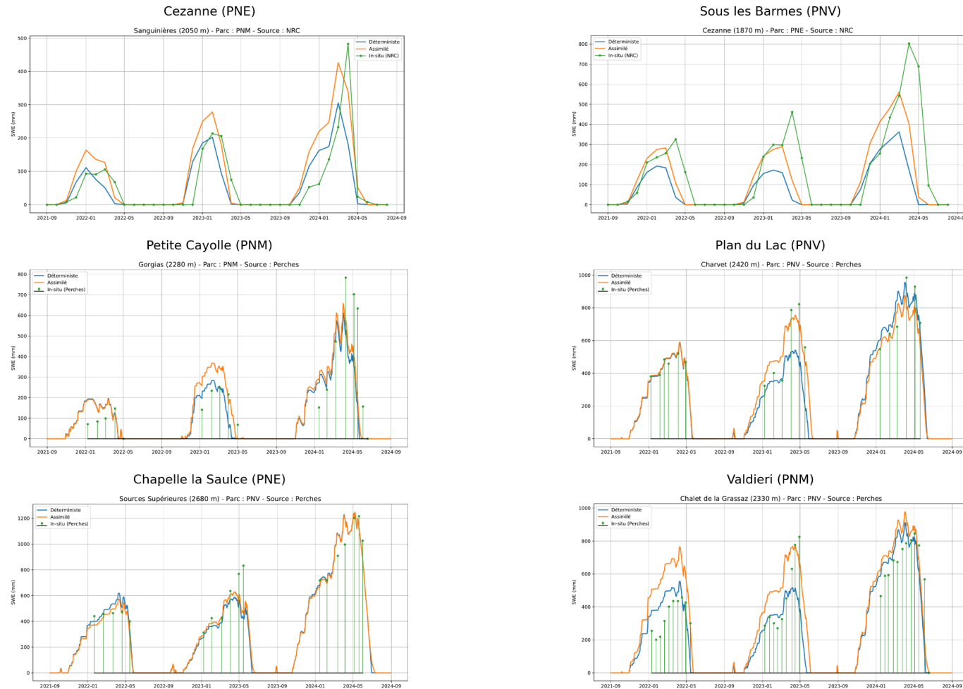
Figure 9 : Seasonal evolution of snow water equivalent (SWE) at selected stations (2021–2024), comparing deterministic and assimilated simulations with in-situ observations.
